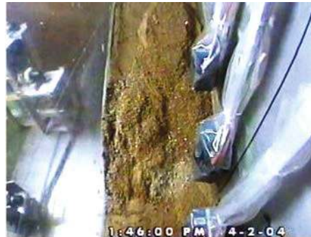
Fig. 23 Top view of the model showing a non-liquefied slide (Ng et al. , 2007)
