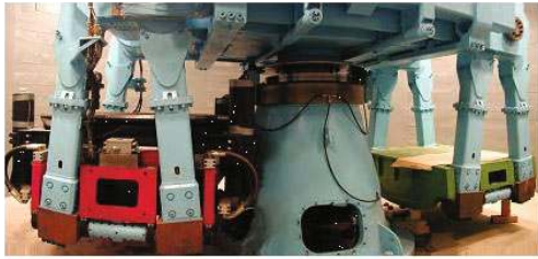
Fig. 4 The 8.5 m-diameter (400g-t) beam centrifuge at HKUST
