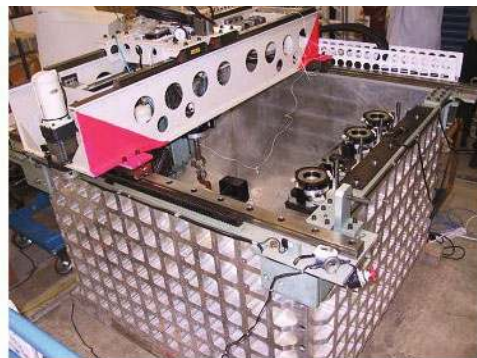
Fig. 6 The four-axis robotic manipulator at HKUST
