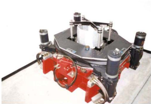
Fig. 5 The bi-axial shaking table at HKUST
