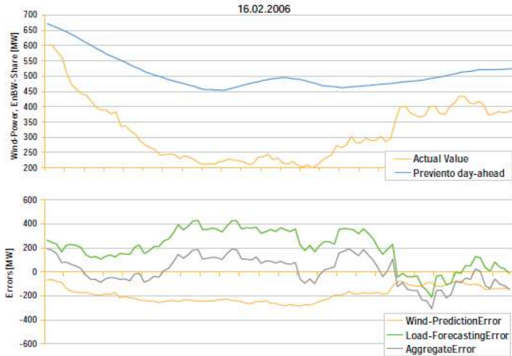
Figure 13: The forecast error for the area of EnBW for the day-ahead forecast of Previento. Source: [53]
