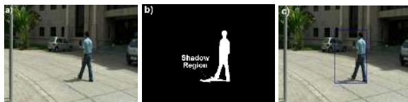
Figure 6: Moving object segmentation for an outdoor scene a) Original frame b) foreground mask c) bounding box representation of object.
