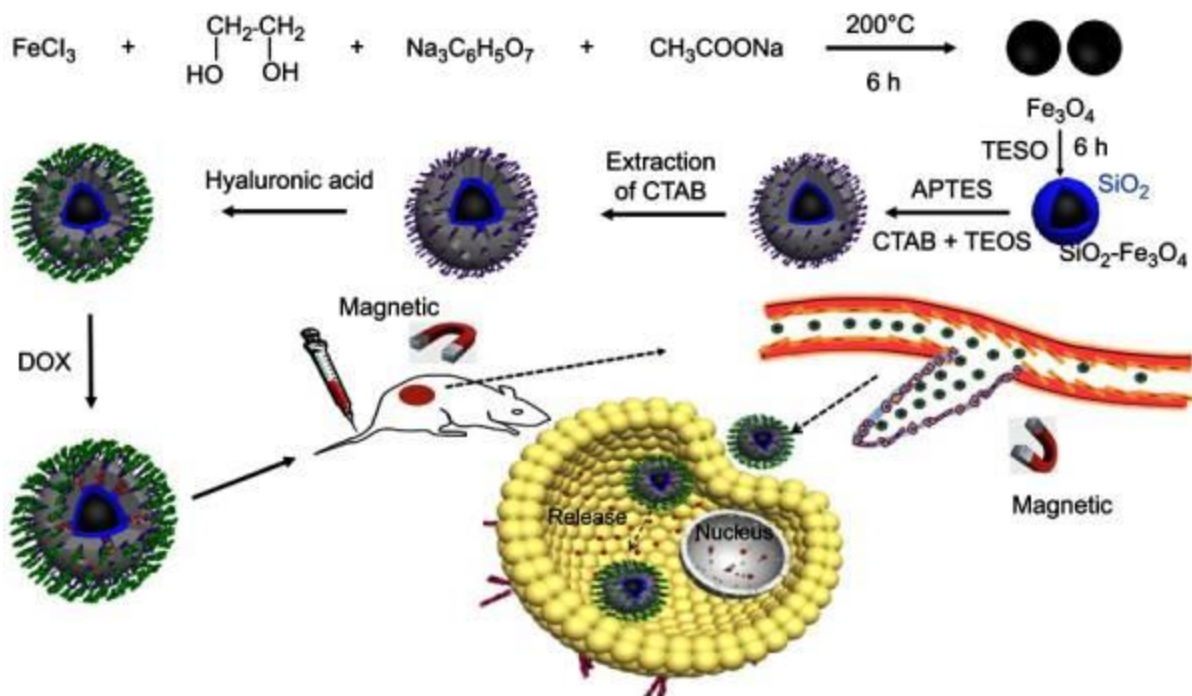
Figure 11. A proposed creation of HA-MSNs for targeted cancer treatment in vivo and pH-responsive drug release following specific binding with cancer cells. Adapted from Fang et al. [95].
