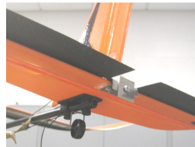
Figure 11. Razor blade fixed to the elevator to sever the perching line.
