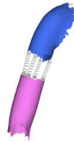
Figure 5. Stitching parts. Parts can be thought of as being connected by springs between the interface points. When the model fits together seamlessly, this stitching cost is zero. During inference, the parts can move apart to fit data and then the inference method tries to infer a consistent model.
