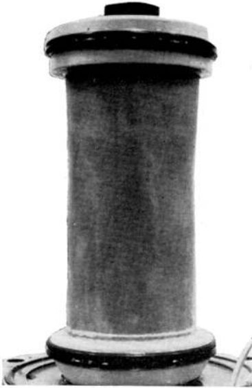
Fig. 6a. 4-in. dia. \times 7-in. high extension test; Ham River sand; porous discs at each end. n_t = 39.2\% , \phi'_{max} = 40.5^\circ , \epsilon_{3f} = -7.4\% , test stopped at \epsilon_3 = -8.4\%
