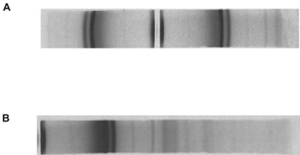
Figure 3. The Guinier pattern of bulk polyethylene. The image of Fourier space of bulk polyethylene was acquired by a focusing camera (Guinier Camera). A- a pattern obtained by the camera with geometrical symmetry. To obtain this image the centre of the camera is placed in the path of the rays ( 2\theta = 60^\circ ). B- a pattern obtained by a non-symmetrical camera ( 2\theta = 0 to 2\theta = 100 ). Due to the high dispersion x-ray pattern one gets the impression of observing the x-ray pattern of two different phases at \lambda = 1.54 \text{ \AA} . The fine diffracted lines at small angle hidden in background are clearly seen in Figure 7F. doi:10.1371/journal.pone.0006228.g003
