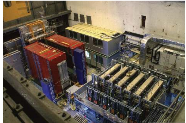
FIGURE 13: Photograph of the CERN hall during the installation of the CHORUS (bottom right) and NOMAD (top left) detectors along the WANF muon neutrino beam.
