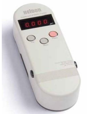
Fig 2.3.1.1 Optical image of 94i-II The Hiedon 94i-II measur the static friction coefficient.
