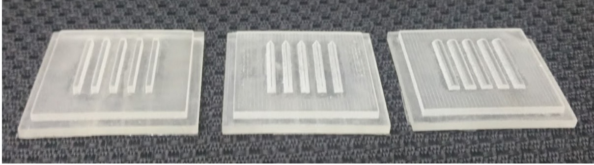
Fig 3.3.2 Optical image of the three different textures. The textures were designed to be removable and the textures were mounted on a linear stage for sliding experiments
