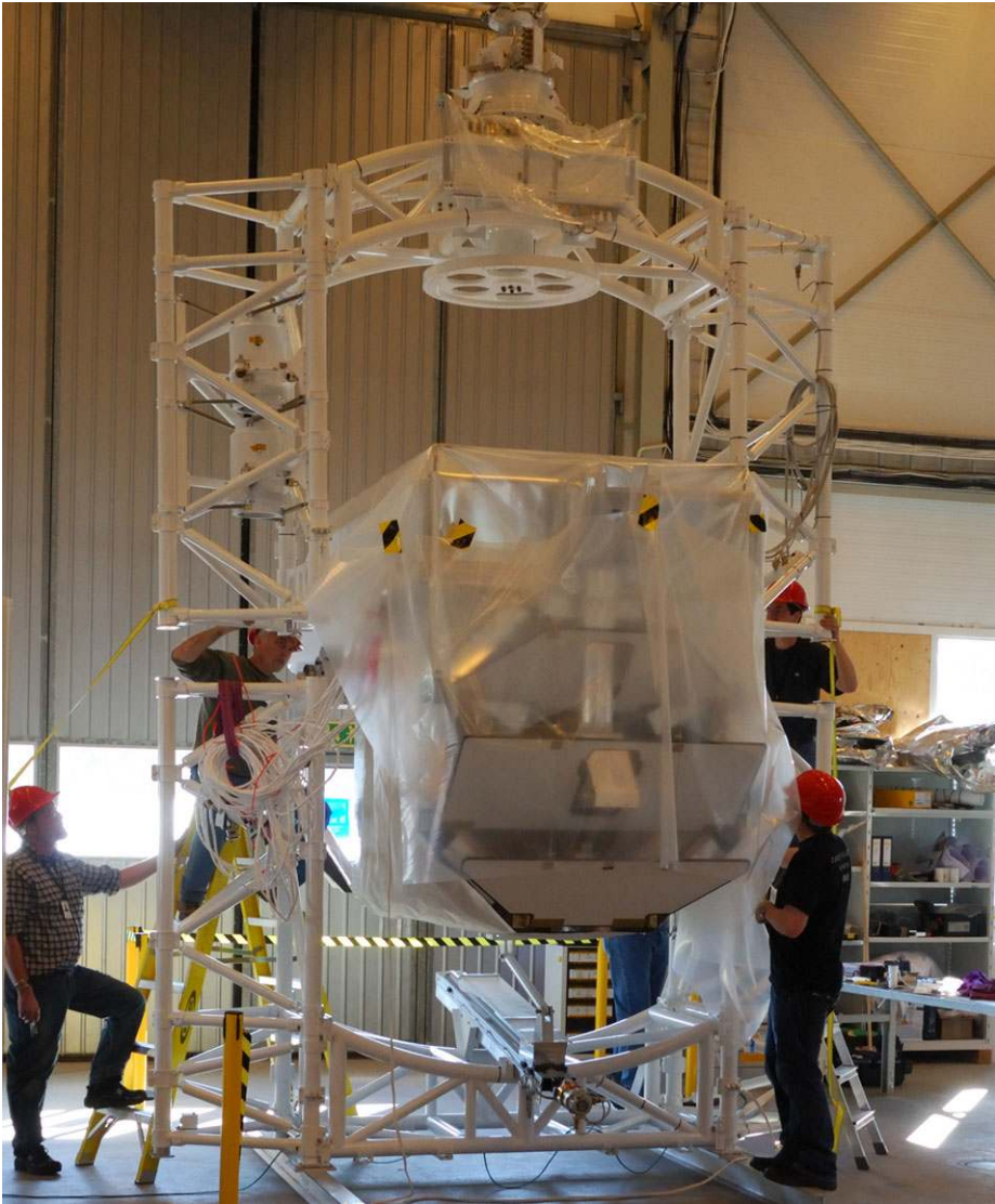
Figure 10 Sunrise gondola main structure during integration of the science payload. The two cylinders in the upper left side truss contain the science data storage systems.
