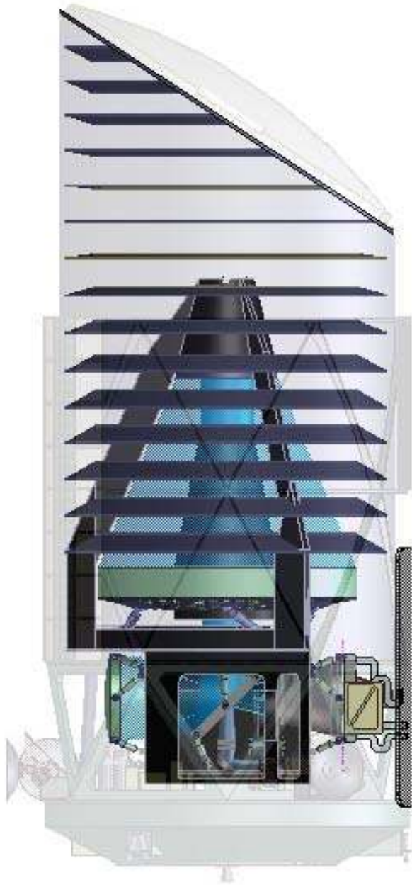
Figure 17 — Schematic treatment of the outer baffle interior vane arrangement. Sunlight is incident from the left, where the height of the baffle and its angled forward edge maintains the baffle interior in darkness. Earthshine is at times incident from the right, however, and therefore the vane angles require particular attention so that the lower vane surfaces are not illuminated by the Earth.
