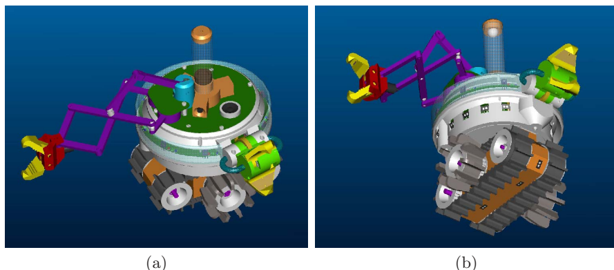
Fig. 2. Graphic visualisation of the s-bot concept. (a) The main body (turret), which has a diameter of 116 mm, is equipped with passive and active gripping facilities, sensors and electronics. (b) The lower body (traction system) is equipped with tracks and hosts the batteries.
