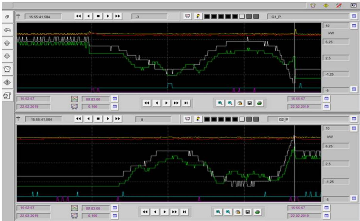
Fig. 8. Process of failed synchronization when using standard control algorithms
