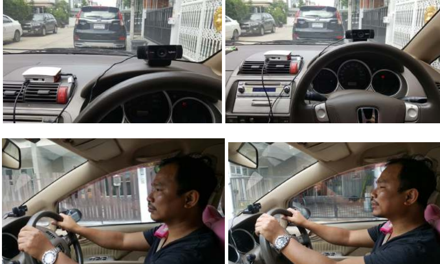
Fig. 18. Fatigue Monitoring System Installation
