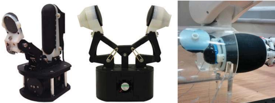
FIG. 2. The TacTip-M2 integrated into the open-hand model M2 gripper ( left ), the TacTip-GR2 mounted on the GR2 gripper ( middle ), and the TacCylinder in a simulated tumor detection experiment ( right ).
