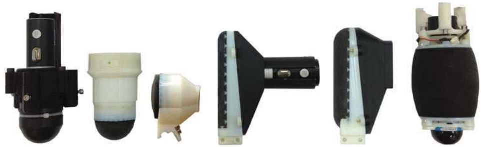
FIG. 1. TacTip project sensors. From left to right : open-TacTip (original), TacTip (improved), TacTip-GR2, TacTip-M2 (flat), TacTip-M2 (round), and TacCylinder.
