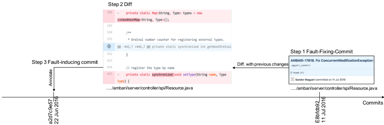
Figure 1: An example of the execution of the SZZ algorithm.
