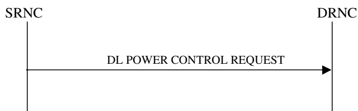
Figure 25: Downlink Power Control procedure, Successful Operation
