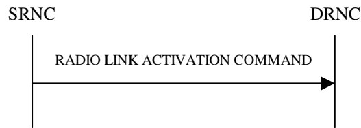
Figure 26D: Radio Link Activation procedure
