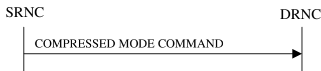
Figure 26: Compressed Mode Command procedure, Successful Operation
