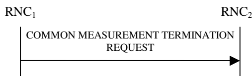
Figure 30D: Common Measurement Termination procedure, Successful Operation
