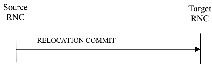
Figure 3: Relocation Commit procedure, Successful Operation
