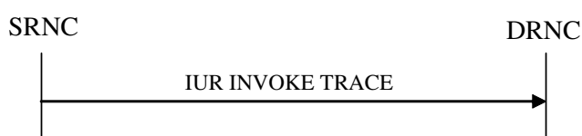
Figure 26K: Iur Invoke Trace procedure, Successful Operation
