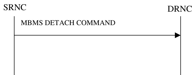
Figure 32: MBMS Detach procedure, Successful Operation
