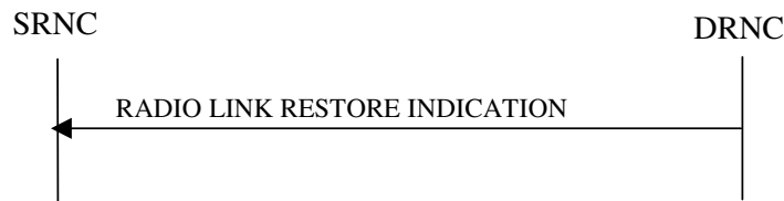
Figure 19: Radio Link Restoration procedure, Successful Operation
