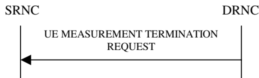
Figure 26I: UE Measurement Termination procedure, Successful Operation
