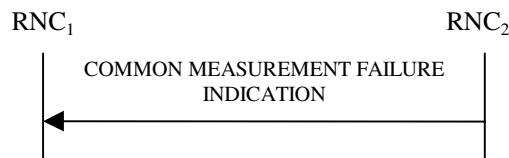
Figure 30E: Common Measurement Failure procedure, Successful Operation
