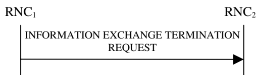
Figure 30I: Information Exchange Termination procedure, Successful Operation
