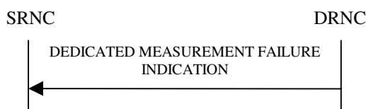
Figure 24: Dedicated Measurement Failure procedure, Successful Operation
