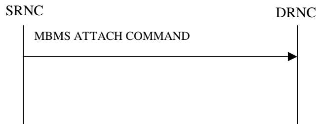
Figure 31: MBMS Attach procedure, Successful Operation
