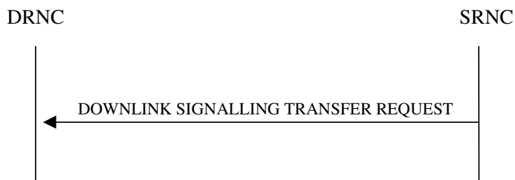
Figure 2: Downlink Signalling Transfer procedure, Successful Operation
