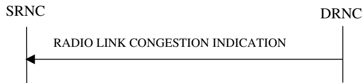
Figure 26C: Radio Link Congestion procedure, Successful Operation
