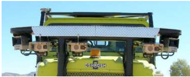
Figure 10. The SICK LIDARs and the cameras are placed on a rigid bar onto the vehicle hood.
