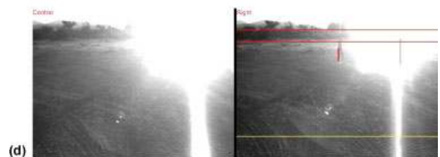
Figure 16. Images captured at sunrise, representing the view with (a) and without (b) the developed camera gain control scheme; (c) and (d) show the result of obstacle detection in bad illumination conditions: although a part of the images are oversaturated, the terrain is visible and the algorithm can be run; obstacles can be detected until they enter the oversaturated area.
