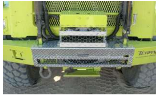
Figure 12. The front of the TerraMax vehicle. Two four-plane laserscanners are visible: the one inside the bumper is the one used during the race, the other (over the bumper) is a backup.
