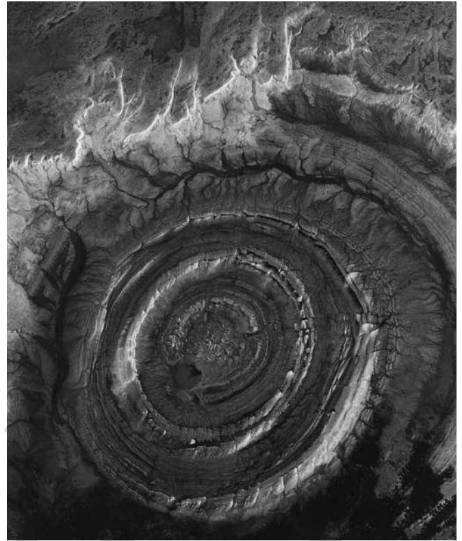
Fig. 10. TerraSAR-X image of the Guelb er Richat ring structure in Mauritania. The image was taken on July 8, 2007; original resolution: 16 m; mode: ScanSAR mode; polarization: VV.
