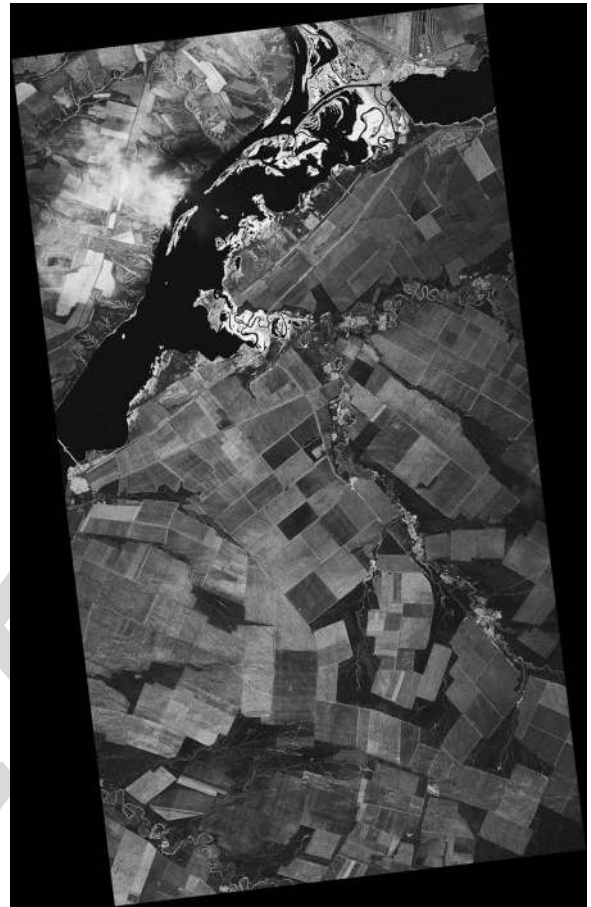
Fig. 6. First TerraSAR-X image, showing a 30 \text{ km} \times 60 \text{ km} area in Russia, western to Volgograd. The scene has been imaged in the stripmap mode, HH polarization, on June 19, 2007. The resolution is approximately 15 m.
