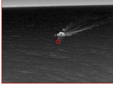
Fig. 6. Example from sequence Boat2 : A report of failure is avoided by increasing the predicted bounding box to the whole image.
