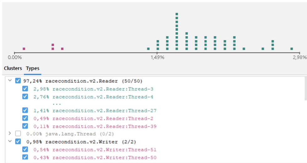
Fig. 11 Histogram for the entire program of the artifact-relative computational runtime of a test case run of Bug 3 with the bug. Here, 50 reader and two writer threads are involved
