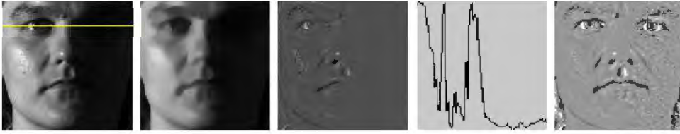
FIG. 6.1. The LTV model. From left to right: f , u^* , v^* , f(20, :) , v' = f/u^* . f(20, :) is the signal along the line depicted in f .
