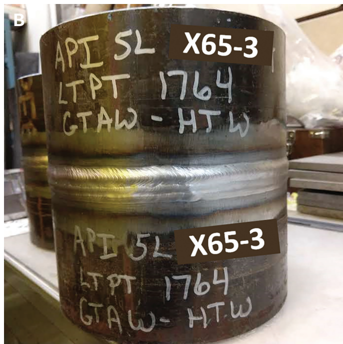
Fig. 1 – A – Example of the weld plates (T17, 46100/1766, GTAW-HW) with the layout for cutting the Charpy impact samples and a metallography sample; B – example of the X65 pipeline weld coupon (X65/1764, GTAW-HW).
