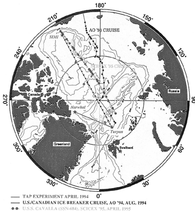
Fig. 1. Transmission paths of the TAP experiment. The AO'94 icebreaker cruise and the SCICEX'95 submarine transect. The black dots on the Turpan/SIMI path are the SVP locations used in the modeling.
