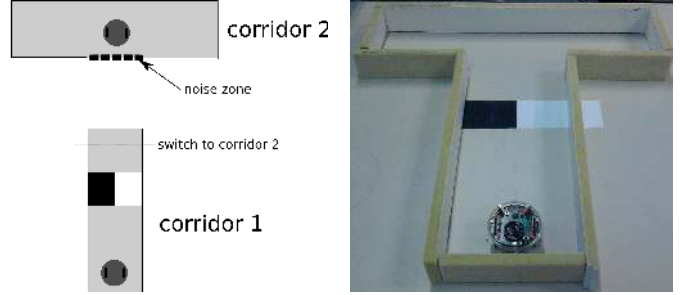
Fig. 9. Left, representation of the T-maze used as minimal simulation; right, photography of the real T-maze with both color patterns
