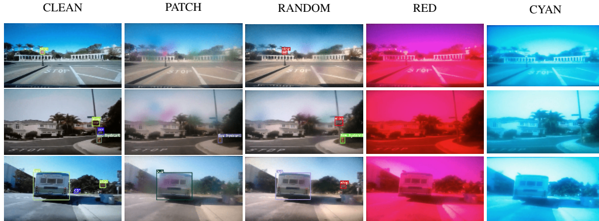
Figure 5: Examples of frames presented to the detection model and its detections when various patches are applied to the camera’s lens. Each row represents a single frame, and each column represents the use of a different patch.
