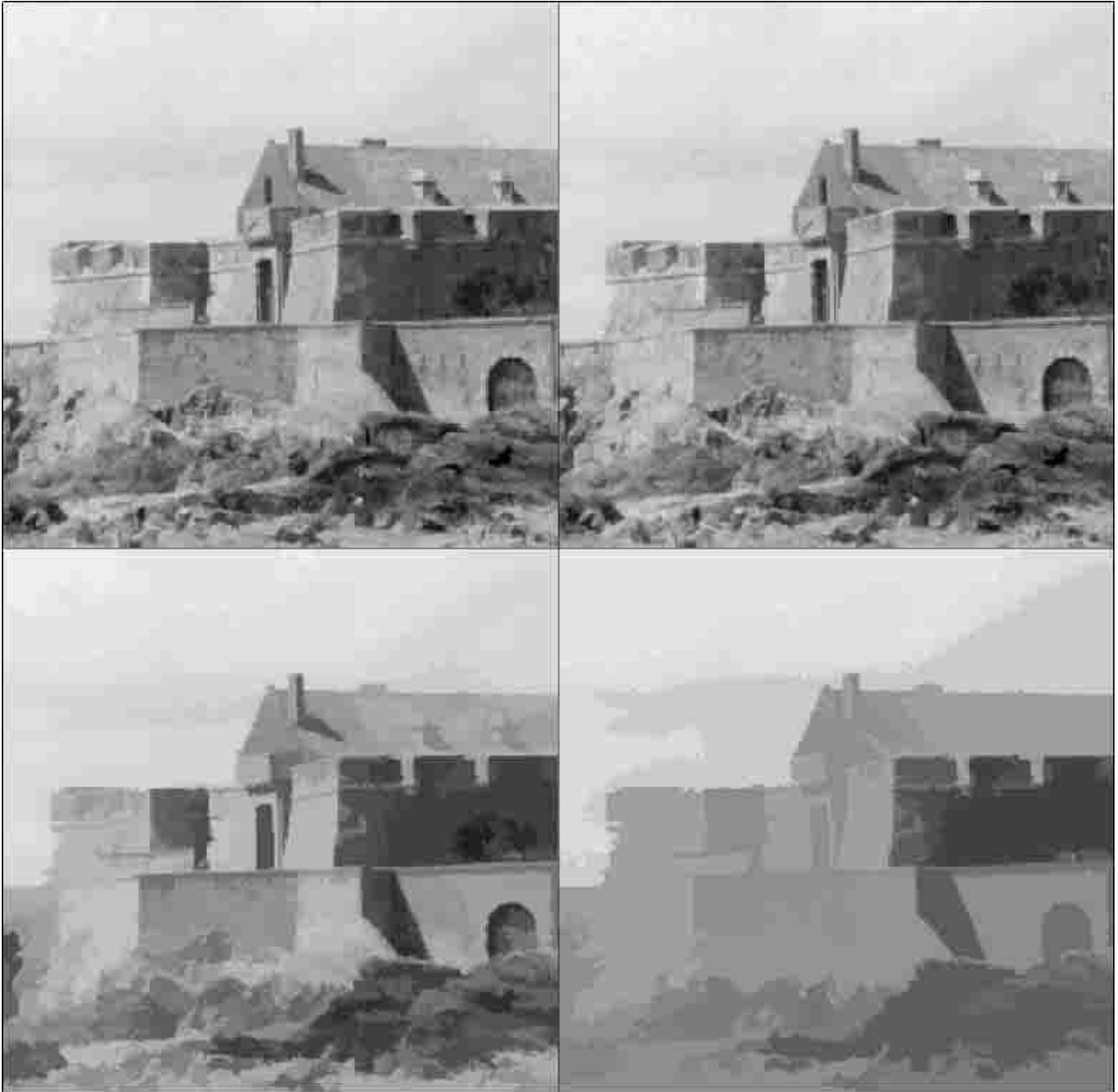
FIGURE 4. Effect of the adaptive quantization on an image of size 500 \times 500 . From left to right, top to bottom: a = 1 (8,834 sections), a = 20 (1,938), a = 400 (155) and a = 8,000 (18).
