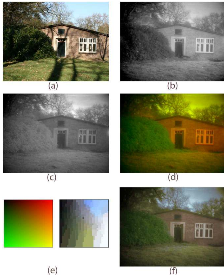
Fig 3. Color remapping procedure. (a) Daylight color reference image. Visible (b) and NIR (c) images of the same scene as in (a). (d) Two-band (RG) false-color image obtained by assigning (b) to the green and (c) to the red channel of an RGB color image. The blue channel is set to zero. (e) The color mapping derived from corresponding pixel pairs in (a) and (d). (f) Result of the application of the mapping scheme in (d) to the false-color image in (d).
