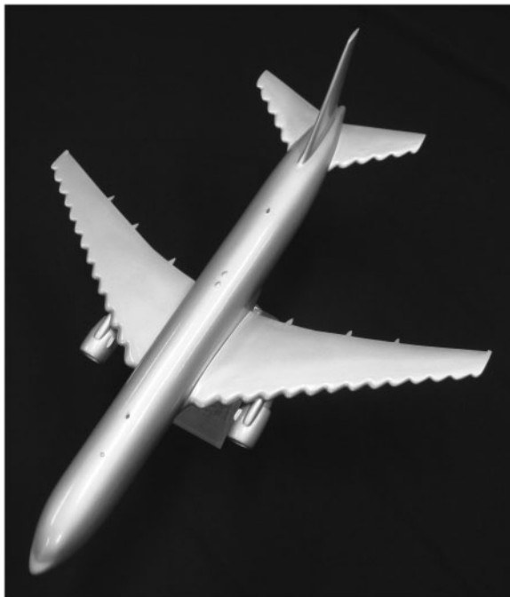
Fig. 8 Model of commercial jet airliner with leading-edge tubercles on the wings and stabilizers. Addition of tubercles on wings could potentially improve safety and reduce weight and fuel costs by the removal of control surfaces needed to change the stall characteristics of the wings.
