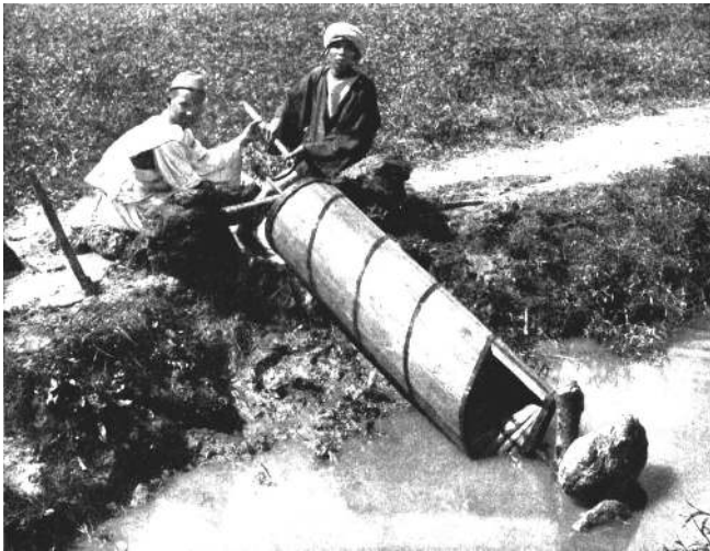
FIG. 3. Two-Bladed Archimedes Screw in Use in Modern Times in Egypt to Irrigate Fields
