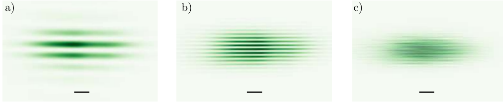
Figure 4.13: Examples of vertical lattices created using the optical accordion set-up proposed in [74]. Light intensities of lattices with spacing (a) 11\ \mu\text{m} , (b) 3.6\ \mu\text{m} and (c) 1.2\ \mu\text{m} . Scale bars indicate a distance of 20\ \mu\text{m} on the atoms.
