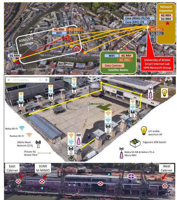
FIGURE 2. UoB test-bed: (a) fibre and radio connectivity (b) millennium square test-bed (c) M-shed museum.
