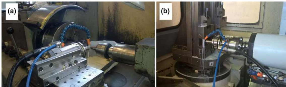
Fig. 2 a The ultrasonic burnishing equipment installed into a manual lathe. b The equipment installed in NC machining centre
