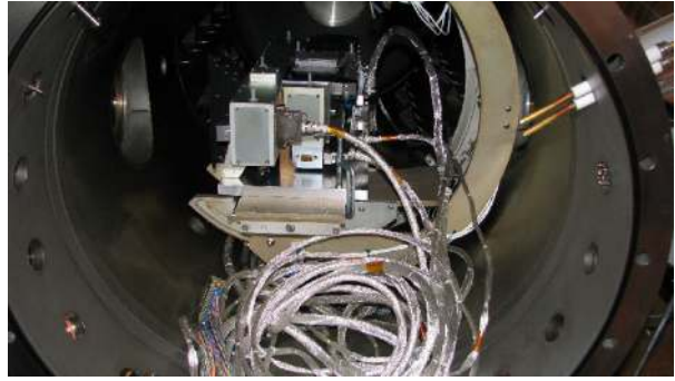
Fig. 7 Juno-UVS just prior to undergoing testing in SwRI's vacuum radiometric calibration facility
