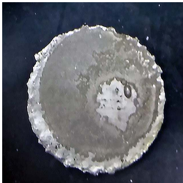
Figure S8. Optical images of the lithium metal anode extracted from the cell containing PMTH cathode after 100 cycles. Mossy and uneven Li deposition including dendrite formation leading to premature cell failure can be visibly observed.
