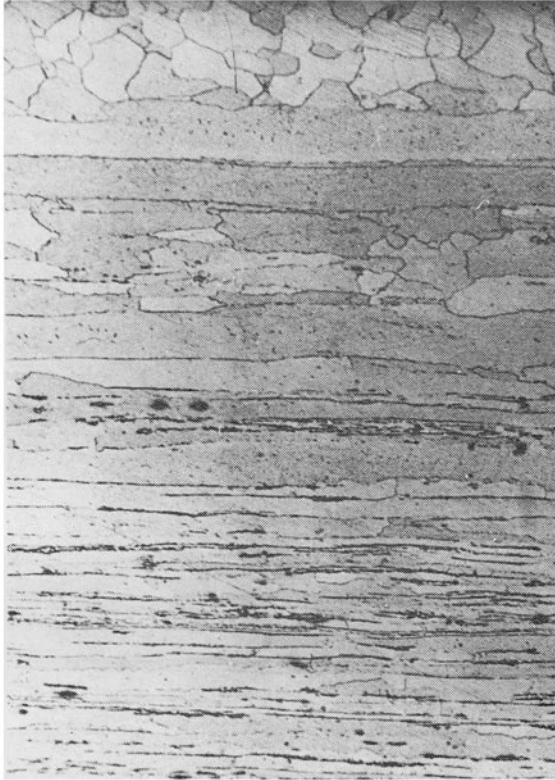
Figure 12. Longitudinal section micrograph (surface to centre) of hot-rolled strip of regular material, 100 × (Mishra et al 1984a).
