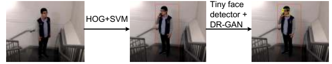
Fig. 14. The UCIA working flowchart. The red bounding box denotes a detected calling/talking motion, whereas the yellow bounding box denotes a detected user face.
