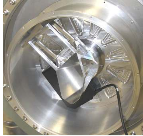
Fig. 4. Derotator consisting of three high quality optical flat mirrors, mounted on a rotation stage, can compensate for the sky rotation to keep the array pattern in the instrument internal focal plane constant.
