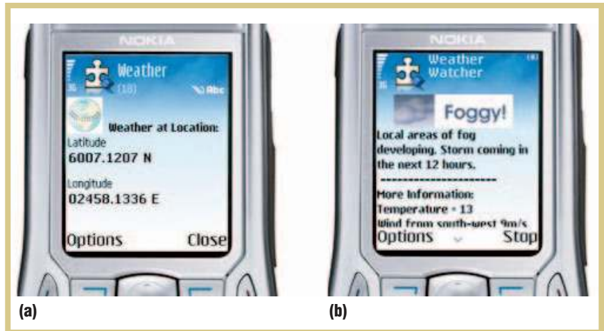
Figure 3. WeatherWatcher using Contory: (a) the user inputs a location of interest. Then WeatherWatcher collects meteorologic observations around this location and (b) displays the infrared weather conditions.
