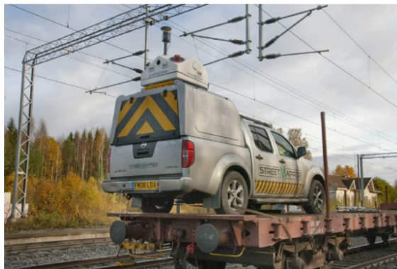
Figure 3. StreetMapper mounted on a train wagon (image from the VR Track Oy [35]).
