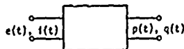
Fig. A1. Two-port electromechanical circuit; e(t) is the voltage at the electrical port, i(t) is the current at the electrical port; p(t) is the pressure at the mechanical port, and q(t) is the volume velocity of the radiating surface.
