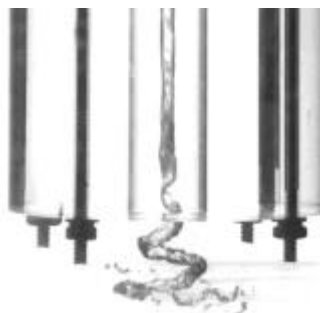
Figure 1: Strobe photograph of plexiglass walled swirling cavitating jet nozzle
