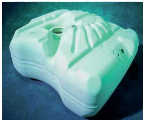
Fuel tank, fully functioning prototype (SLS)
