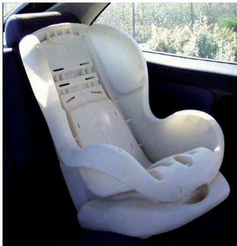
Prototype of a front seat in a car (SLS)
