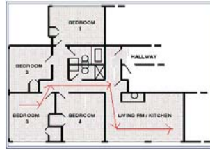
Fig. 2. The movements planner finds a global path from one of the bedrooms to the kitchen
