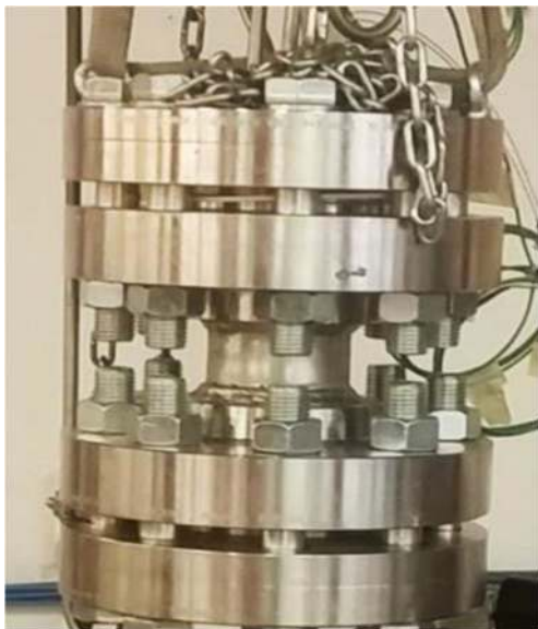
Fig. 1 Image of the reactor used for hydrate formation and \text{CO}_2/\text{CH}_4 replacement into water cages
