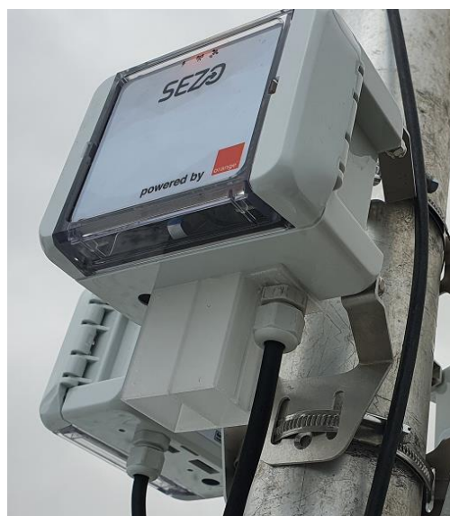
Figure 12. SEZO AM with installed outer sheath of the air inlet (photo from WIRAN resources).
