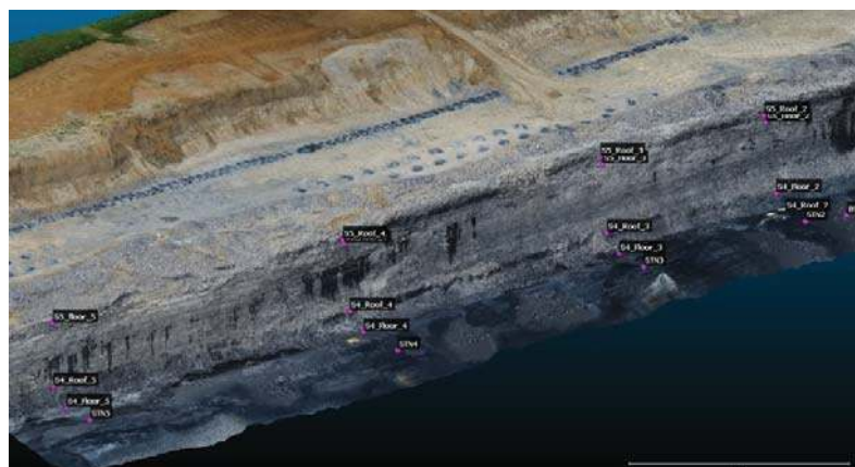
Figure 7—Far South pit mapped no. 4 seam and no. 5 seam contacts with total station points marked (Katuruza and Pretorius, 2018)
