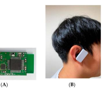
Figure 1. Earbud-type IMU sensor. (A) IMU sensor. (B) IMU sensor attached to the ear.
