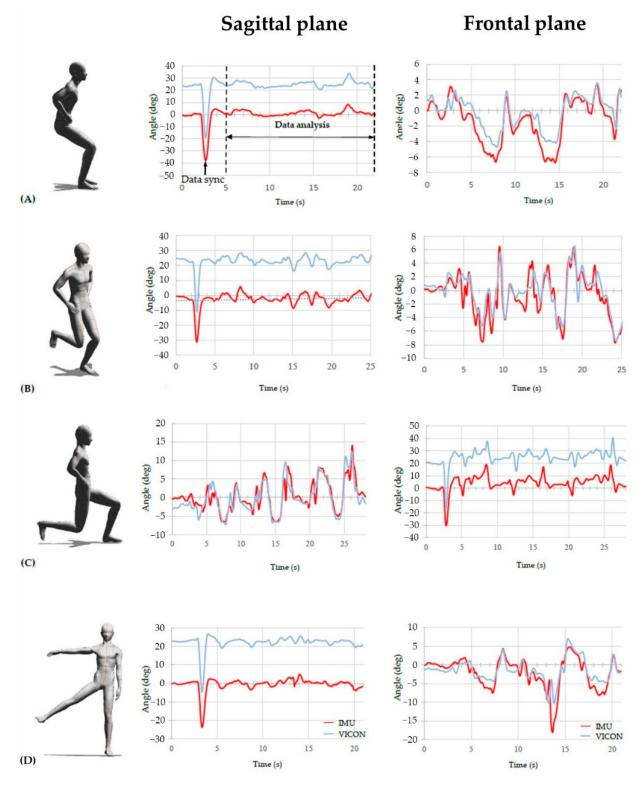
**Figure 2.** Comparisons of head angle between earbud-type IMU sensor and the 3D motion analysis system during each workout in sagittal plane and frontal plane. The two datasets were synchronised with each peak of rapid neck flexion (data sync.): (**A**) squat, (**B**) single-leg squat, (**C**) reverse lunge, and (**D**) standing hip abduction.
